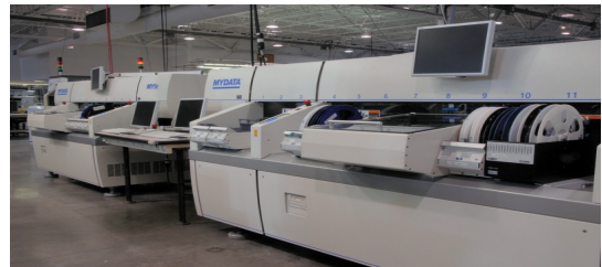
Shown above, Sunburst's new, full-service MYDATA® production line for surface mount applications.
